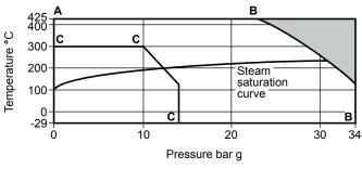
The product must not be used in this region or beyond the parameter of the PMA or TMA of the relative end connection.
